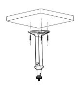
3 Adjust the monitoring angle through nut and universal joint
