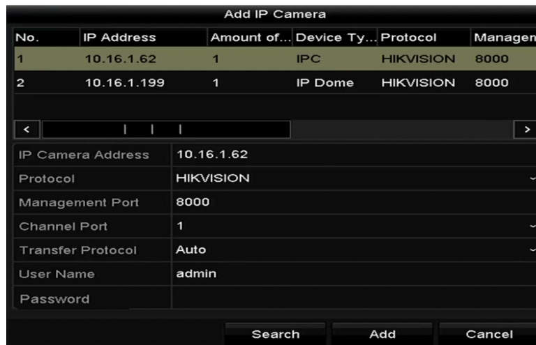
Figure 2-29 Quick Adding IP Camera Interface
