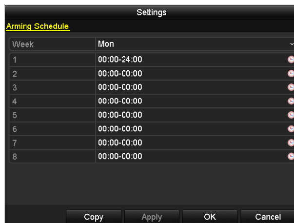
Figure 8-20 Set Arming Schedule of Alarm Output
