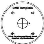
Figure 2-15 Drill Template of the Junction Box
